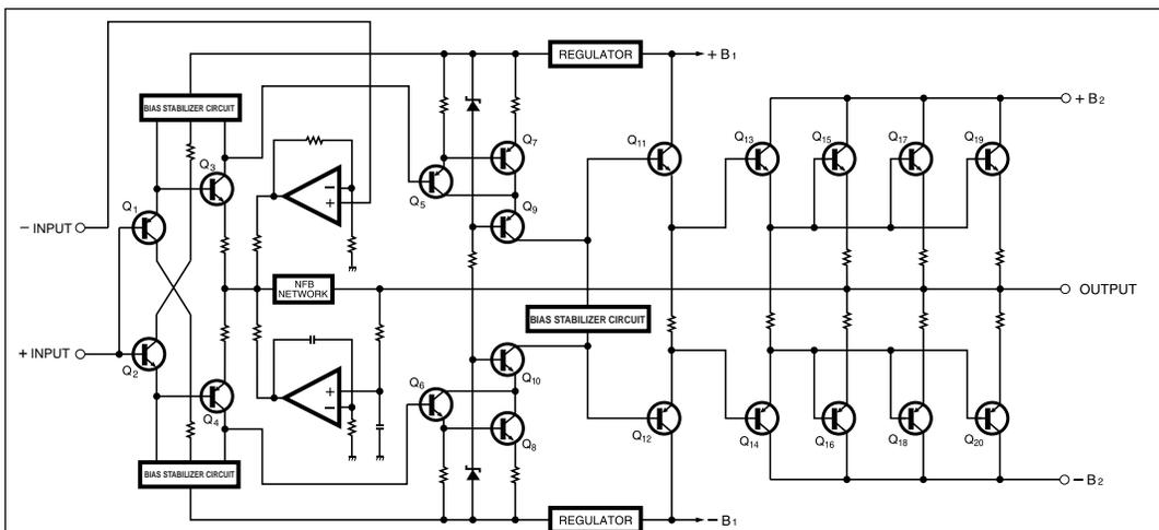
Figure 1 Circuit diagram of amplifier section (one channel)
