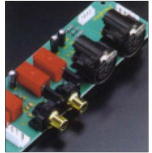
Unbalanced and balanced input connectors
