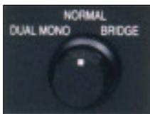
or to obtain the same signal from both speaker outputs for driving a bi-amped speaker setup.
